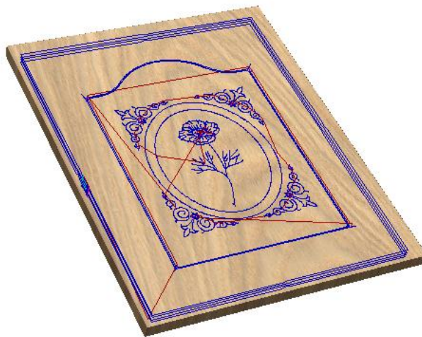
3D Preview showing the calculated toolpaths
