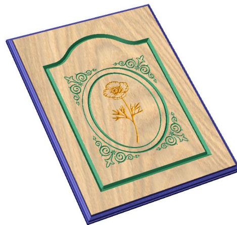
Preview using different colors for each toolpath
