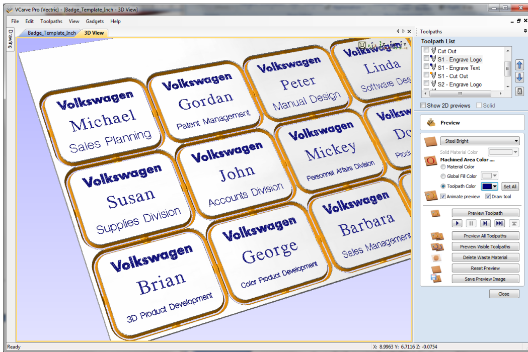
3D window showing the 3 toolpaths for sheet 1
